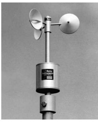
In these anemometers the rotor spindle turns a multislotted disc, interrupting the beam from a lightemitting diode. The output is obtained by amplification of the signal from an opto-electronic sensor in the path of the light beam.
